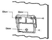
4. Align the Auto-Sync Time Clock with the hooks on the mounting plate. Press down and toward the wall until a "CLICK" is heard. Replace the cover, lock it and remove the key. Your Auto-Sync Time Clock is now wall mounted.
